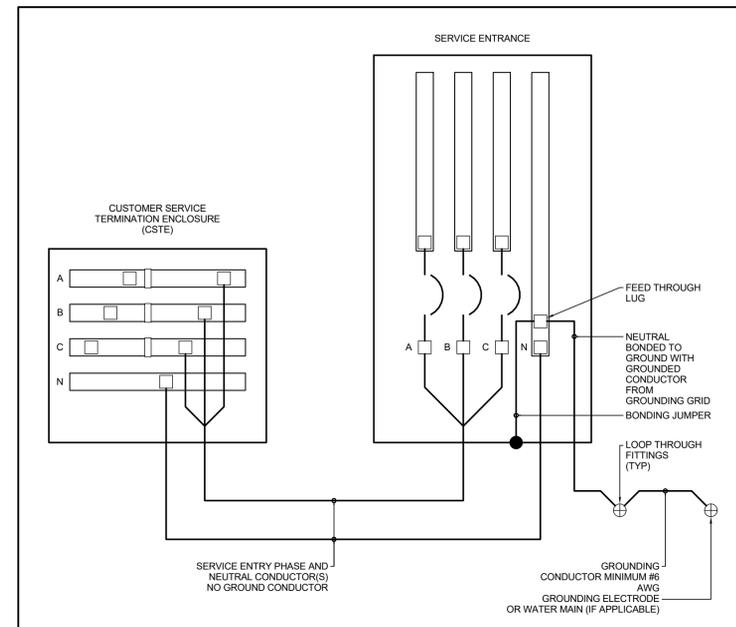
**CSTE WIRING DETAIL - 4 WIRE SERVICE**
